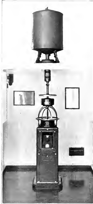
The latest type Kolster radio compass as now being installed on many American merchant vessels.
